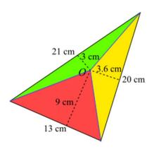
For each smaller triangle, the 'base' and 'height' are shown (the 'bases' are the sides of the original triangle, which are not horizontal). So, using  $Area = \frac{1}{2}base \times height$ , the areas of the smaller triangles can be found:
